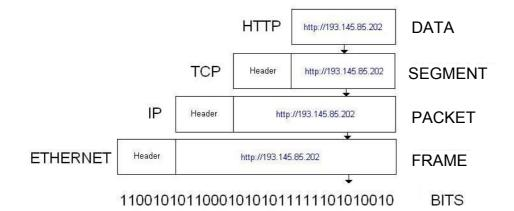
When the encapsulated information arrives at its destination, it must then be deencapsulated. As each layer receives information from the previous layer, it removes the unneeded information contained in the header placed there by the previous layer.
